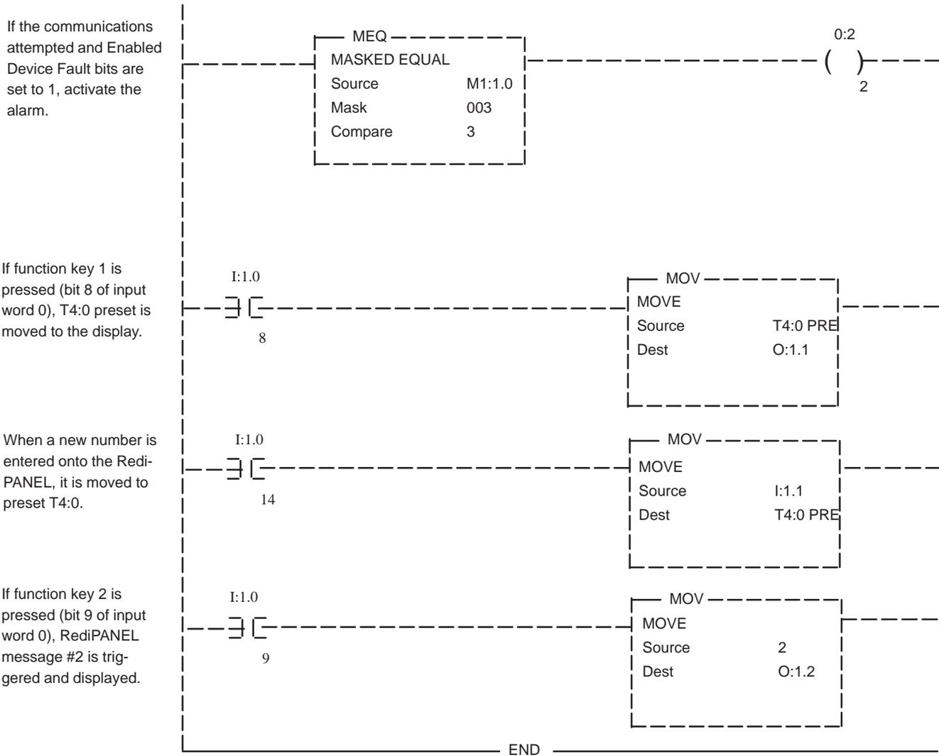
If the communications attempted and Enabled Device Fault bits are set to 1, activate the alarm.
