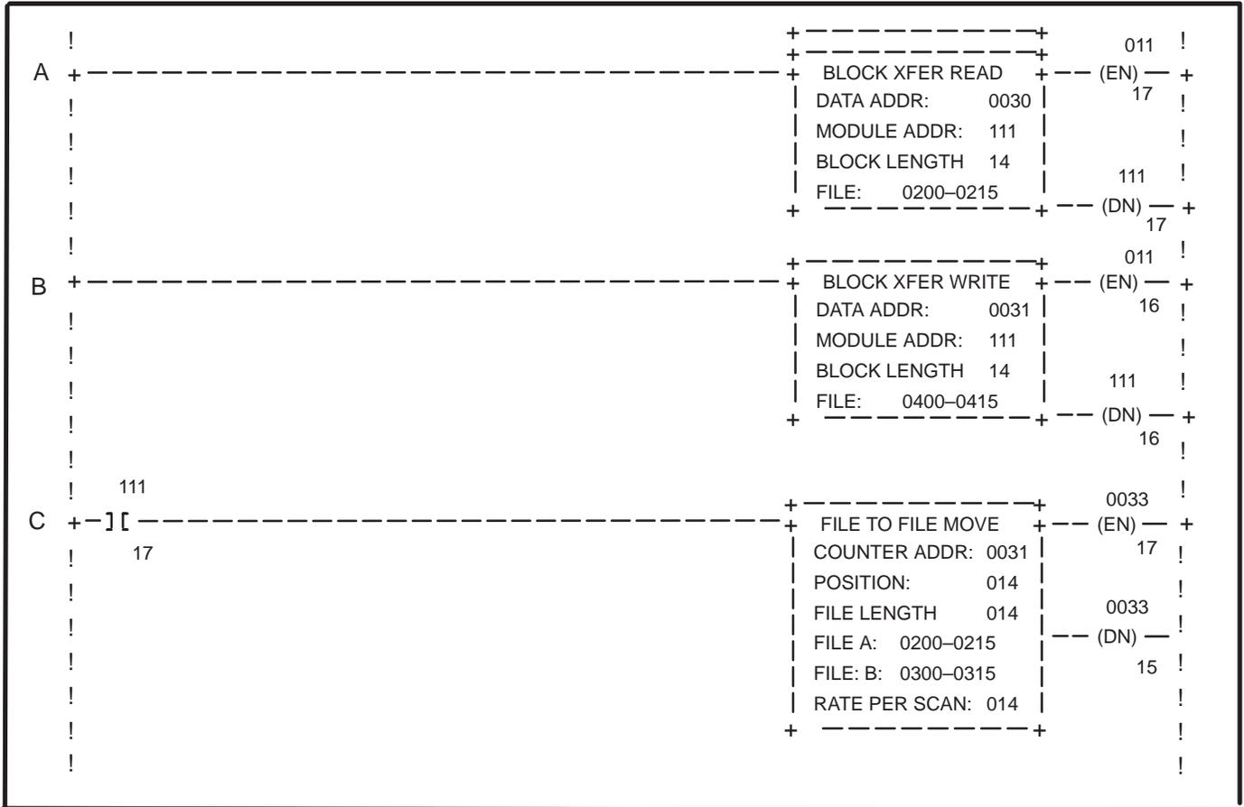
The block transfers and the file-to-file move allow for communications from the sub-scanner to the programmable controller. The block length of 14 allows for 8 utility words needed by the sub-scanner and 6 words (or  $\frac{3}{4}$  rack) for the Keypad Module. The resulting input/output image tables in Figure 7.9, on the following page, go along with this programming example for Keypad Module.
