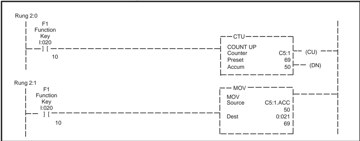
The program example in Figure 7.2 illustrates how the function key, F1, may be used just like a push button or other similar input type device. In this instance, F1 is used to increment the accumulative value of count up counter C5:1 and initiate a MOVE instruction. Each time the F1 function key is pressed, the accumulated value of the counter increases by one and the MOVE instruction moves the new value to the right hand side of the Keypad display.
