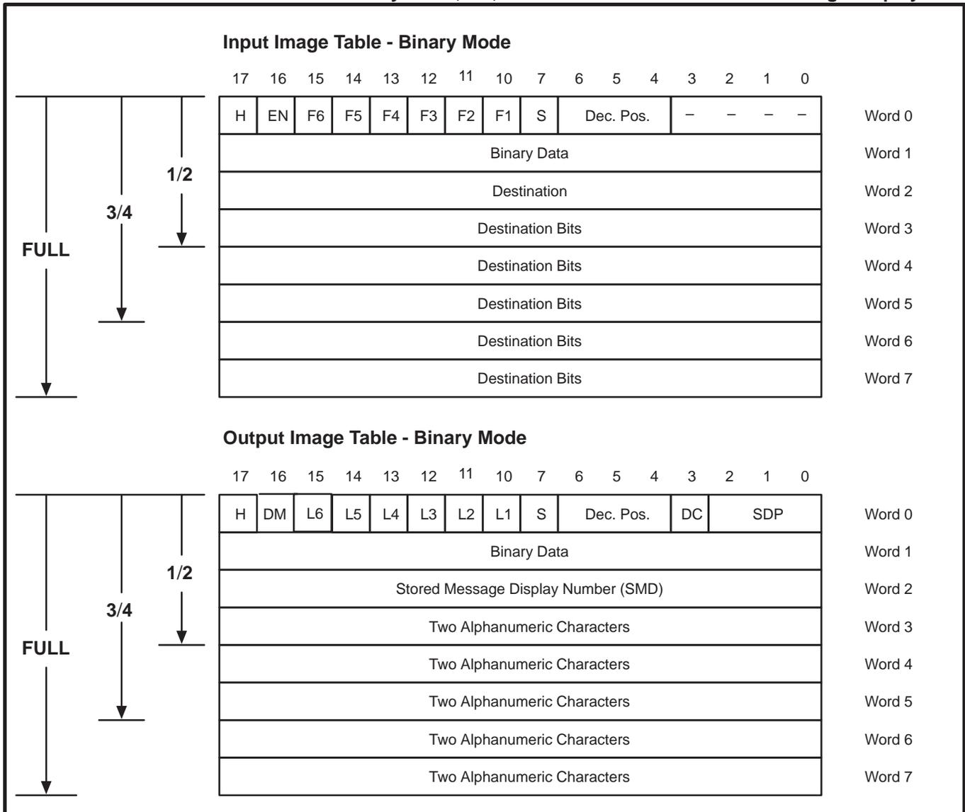
$1/4$  Rack Using Stored Messages    Stored message display cannot be used with  $1/4$  rack configurations.
