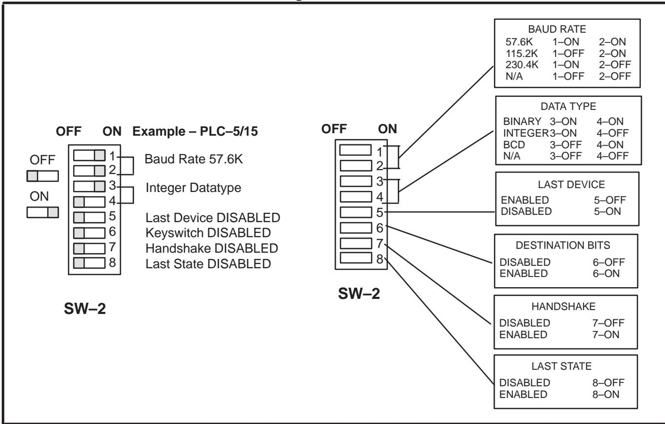
Set BAUD RATE to 57.6K for PLC-5/15 and 5/25 or the module will not communicate with the PLC.
