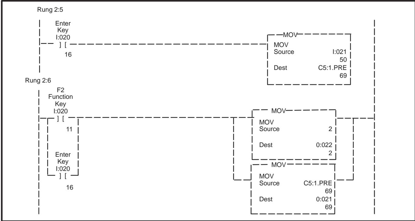
In the example shown in Figure 7.5, rung 2:5 is used to move the value from the input image table, I:021, to counter C5.1 preset, each time the Enter key is pressed.
