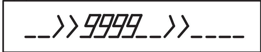
The keypad operator starts by pressing the ENTER key. The present destination is displayed between the >>—>> symbols as shown in Figure 6.3. The flashing >> symbol prompts the operator for a new destination number, followed by another ENTER keystroke. After the second ENTER, the new destination is mapped directly into the destination word.
