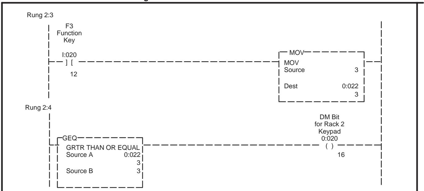
In Figure 7.4, function key F3 is used to initiate a MOVE instruction. The MOVE instruction, moves the constant 3 to the Keypad module's stored message word 0:022. This in turn triggers stored message number 3 "16 CHARACTER MSG."
