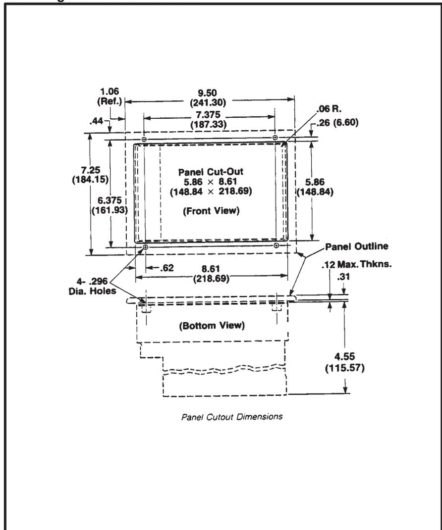
**Step 2** - Drill six 0.312" (7.6mm) diameter holes for the top and bottom mounting brackets. A template is provided with the module to assist in this operation.
