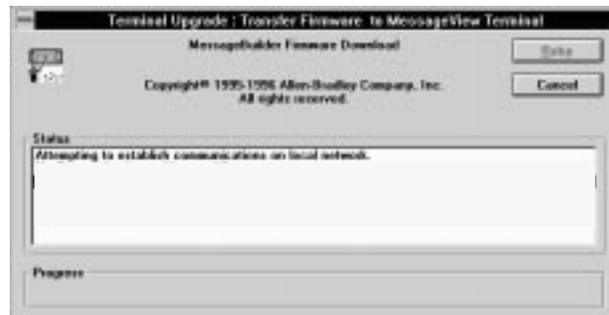
**Note:** The application resident in the terminal was erased as soon as the Firmware Download started. Even if the download is cancelled, the application is gone. If the terminal is switched to Run mode, its startup self-tests will report that there is no valid application.
