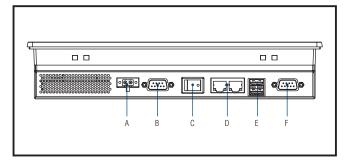
A. DC-in B. RS-232 C. Power S/W D.2 x LAN E. 2 x USB F. RS-232/422/485
