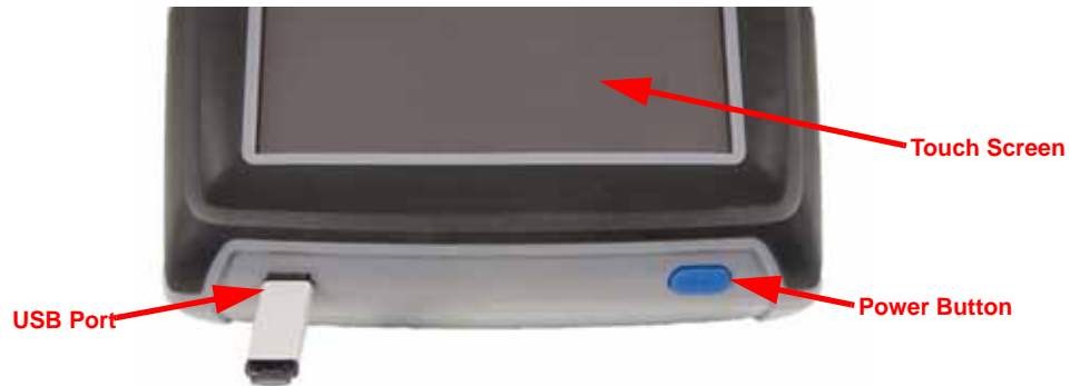
FIGURE 2. Viper Pro Front Panel
