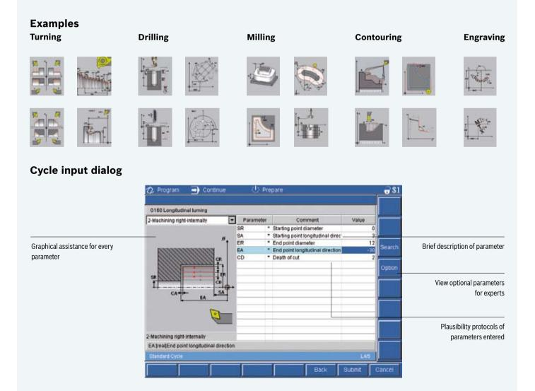
Contour cycles are used to easily program and efficiently machine turning and milling work-pieces. Workpiece contours are described with DIN G-Code and the dimensions for lines, radii and chamfers copied into the program directly from the workpiece drawing. The contour cycles calculate automatic cut segmentation during machining and ensure efficient tool guidance. Threads, grooves, undercuts and pockets are then simply added via parameter configured technology cycles.
