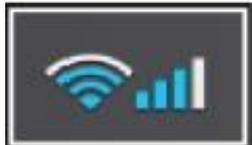
The connectivity top bar icon displays the current signal strength of the Wi-Fi and cellular connection.
