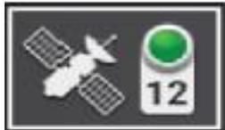
The GNSS top bar icon displays position accuracy status and number of satellites tracked.
