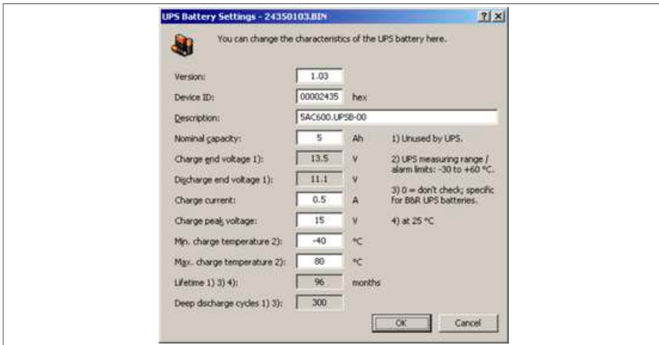
Figure 128: ADI Control Center - UPS battery settings
