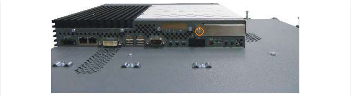
Figure 190: Removing the PCIe module cover
