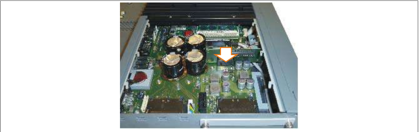
Figure 189: Installing the 5AC803.BC02-00 adapter
