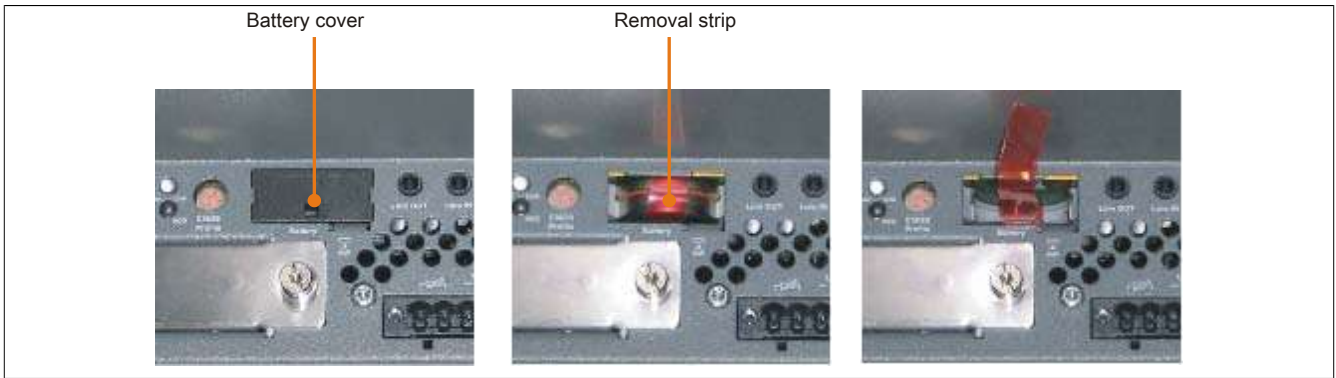
Figure 162: Removing the battery
