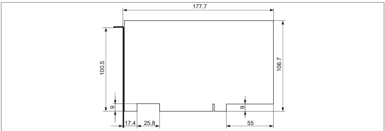
Figure 23: Standard half-size PCI card - Dimensions
