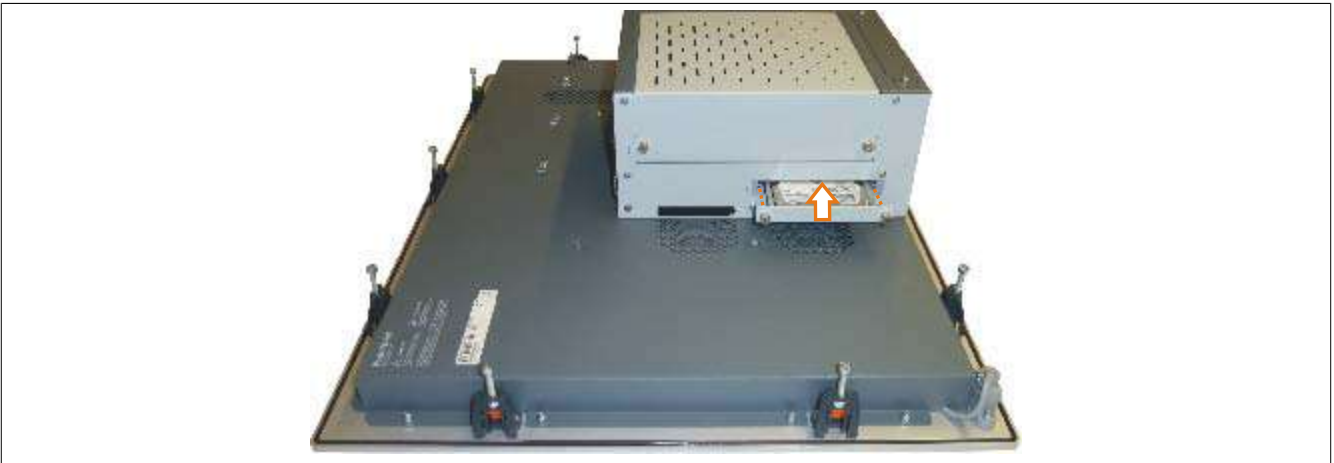
Figure 167: Inserting the compact SATA drive
