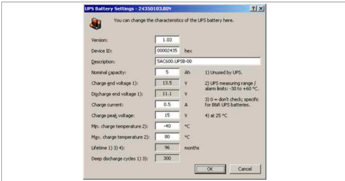
Figure 137: ADI Control Center - UPS battery settings
