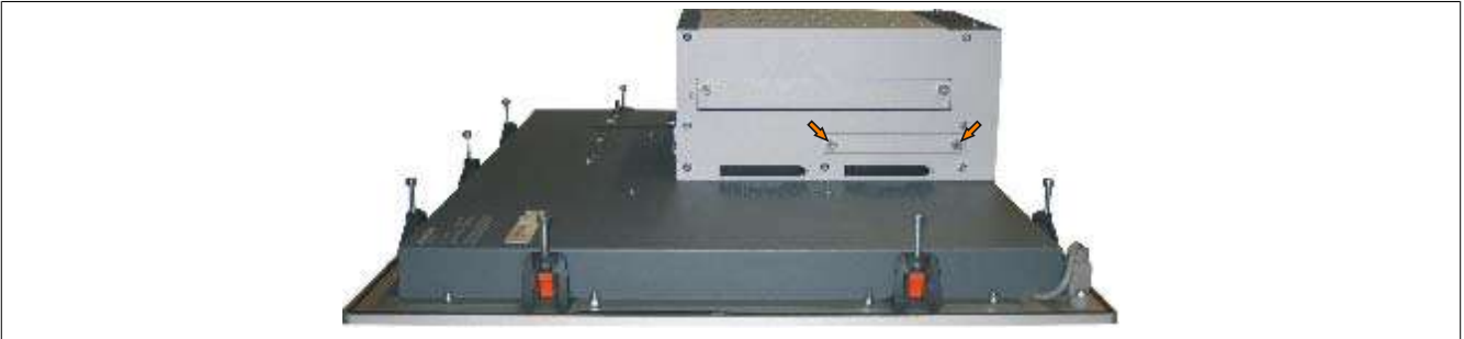
Figure 195: Loosening the quick release screws
