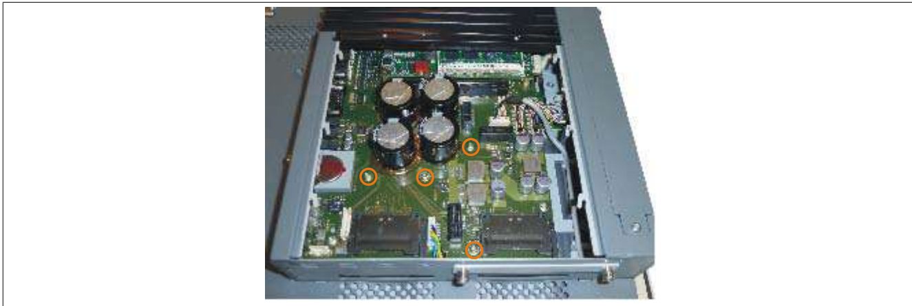
Figure 216: Removing the screws
