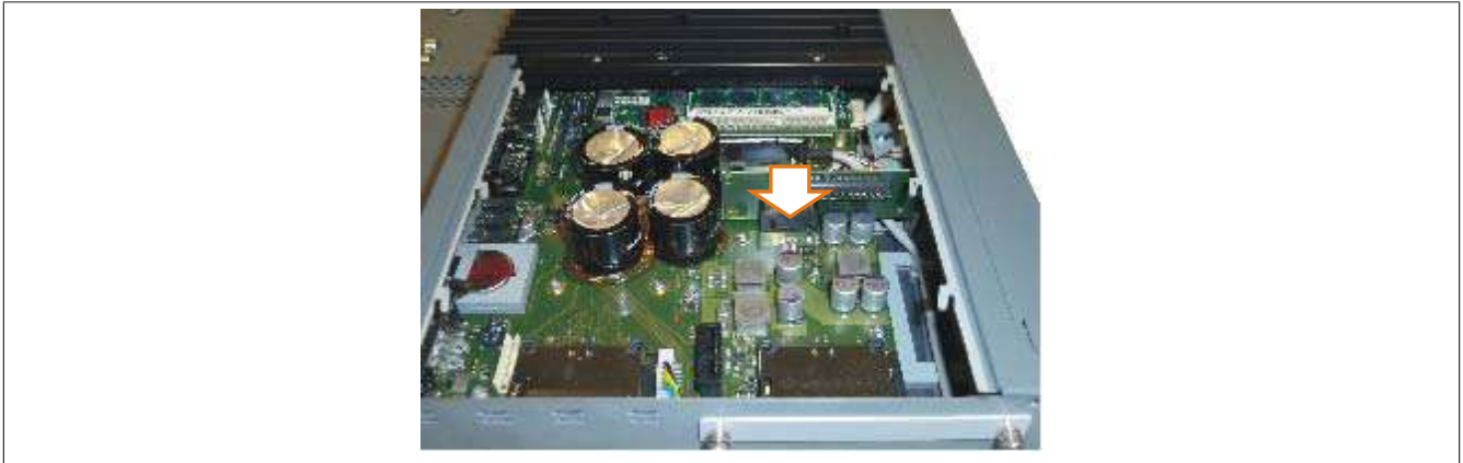
Figure 218: Installing the 5AC803.BC02-00 adapter
