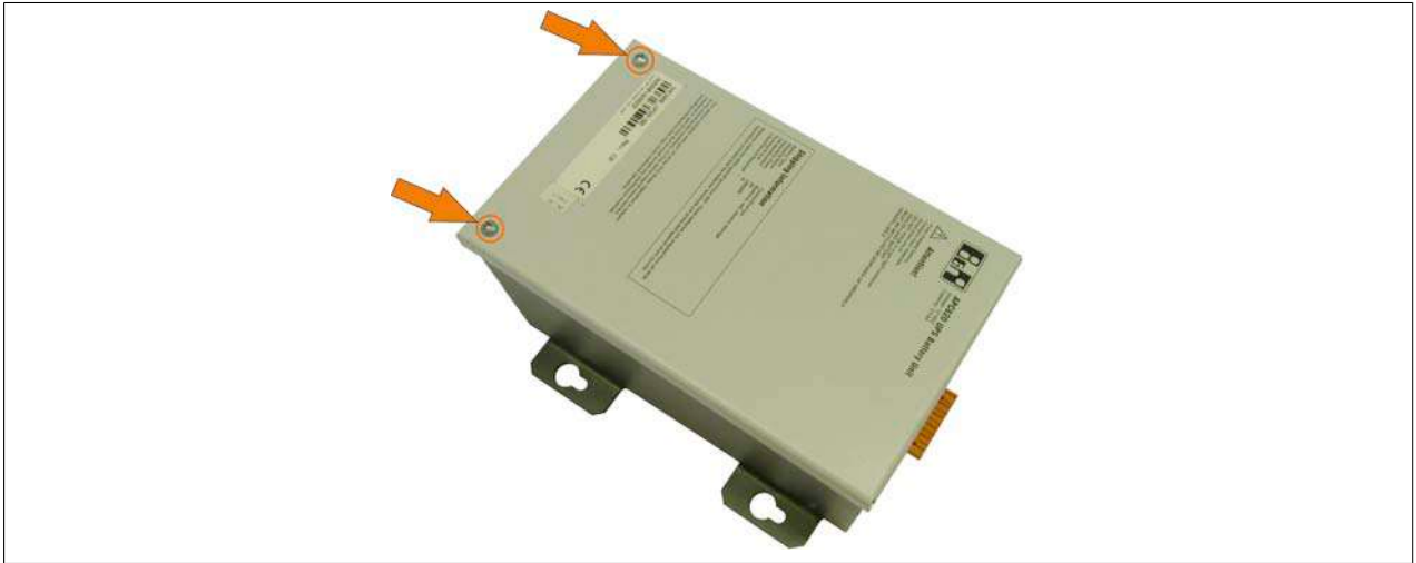
Figure 210: Removing the cover for the battery unit
