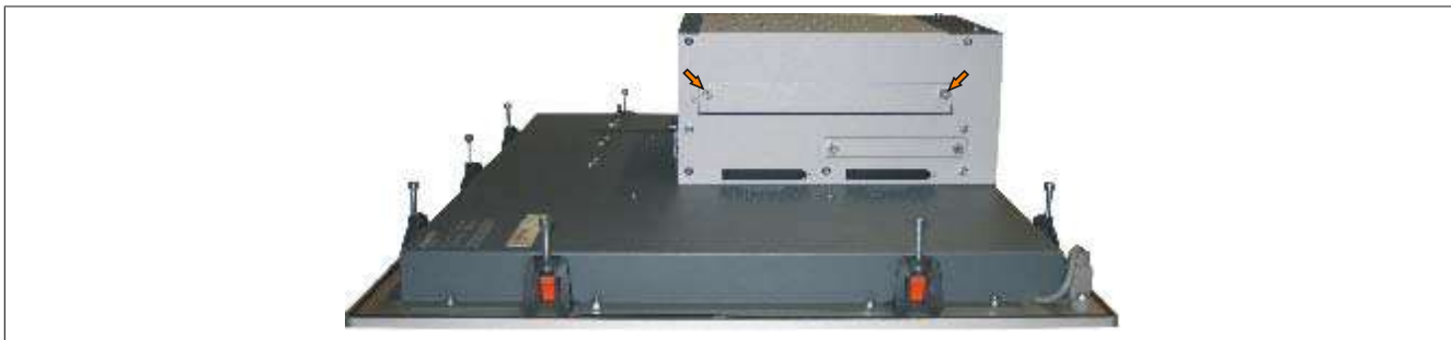
Figure 197: Loosening the quick release screws
