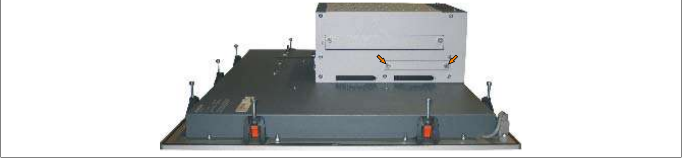
Figure 196: Loosening the quick release screws
