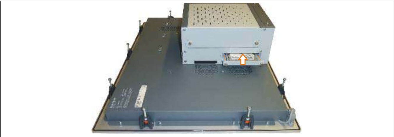
Figure 197: Inserting the compact SATA drive
