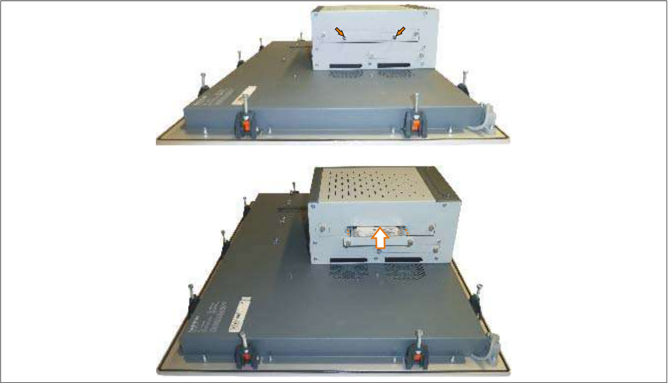
Figure 202: Inserting the slide-in compact drive
