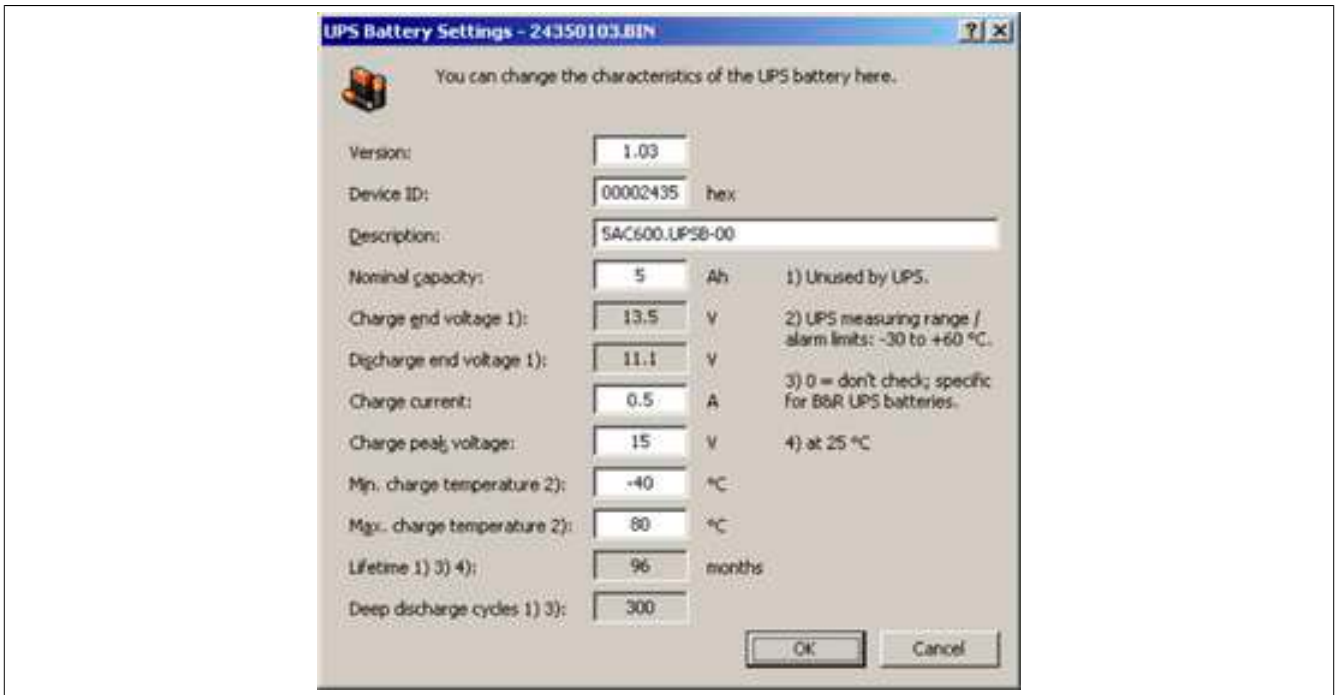
Figure 138: ADI Control Center - UPS battery settings
