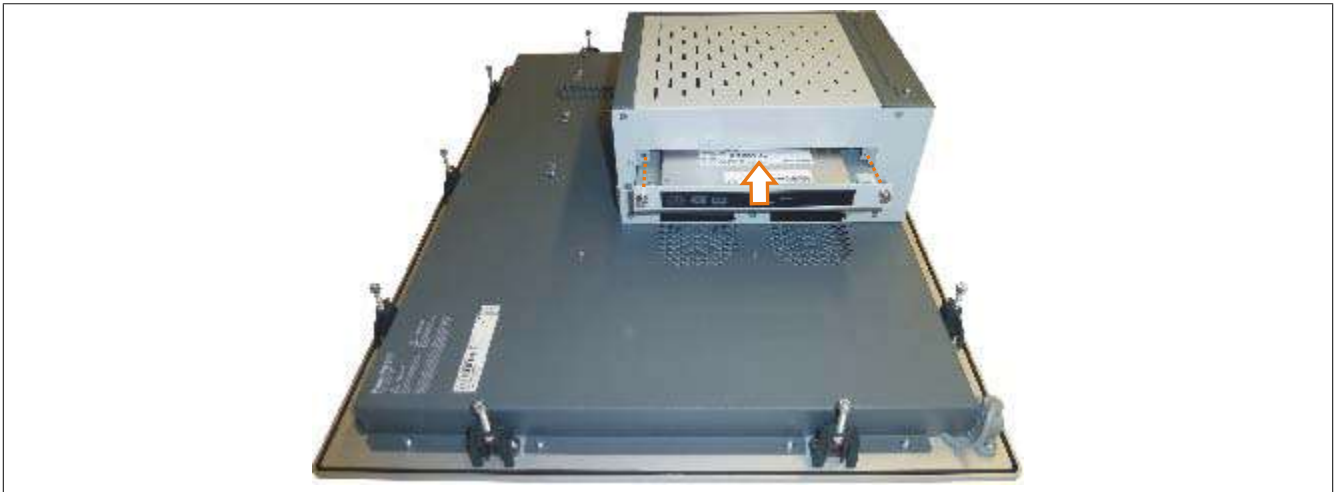
Figure 199: Installing the slide-in drive
