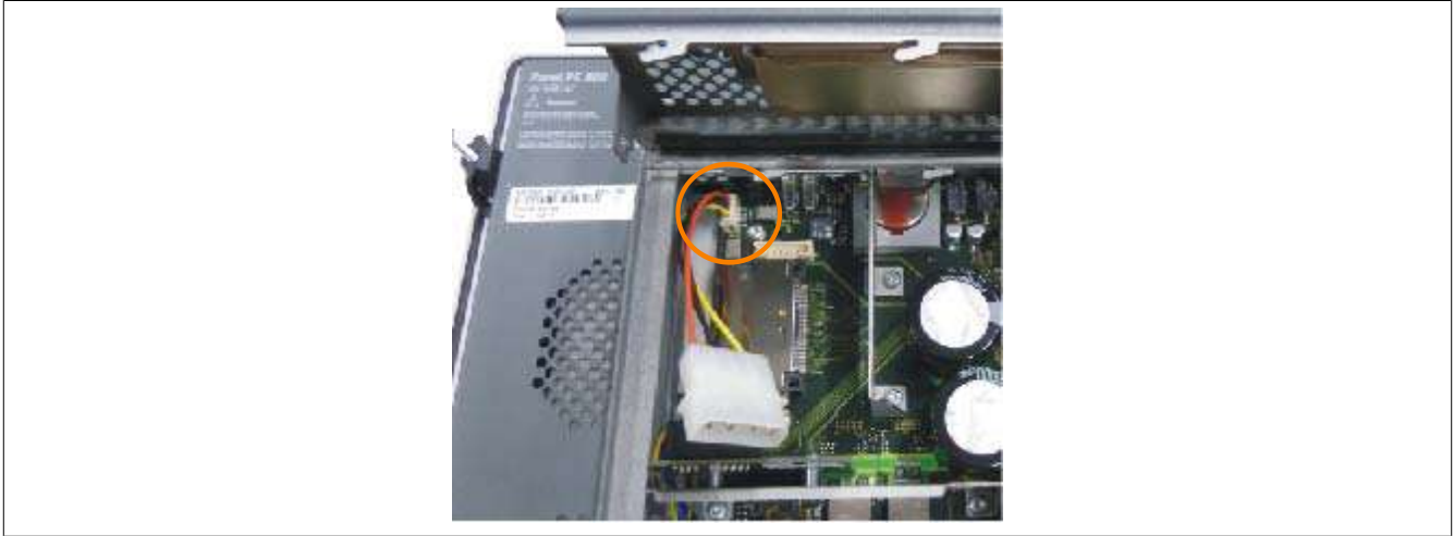
Figure 227: Connector location for external devices
