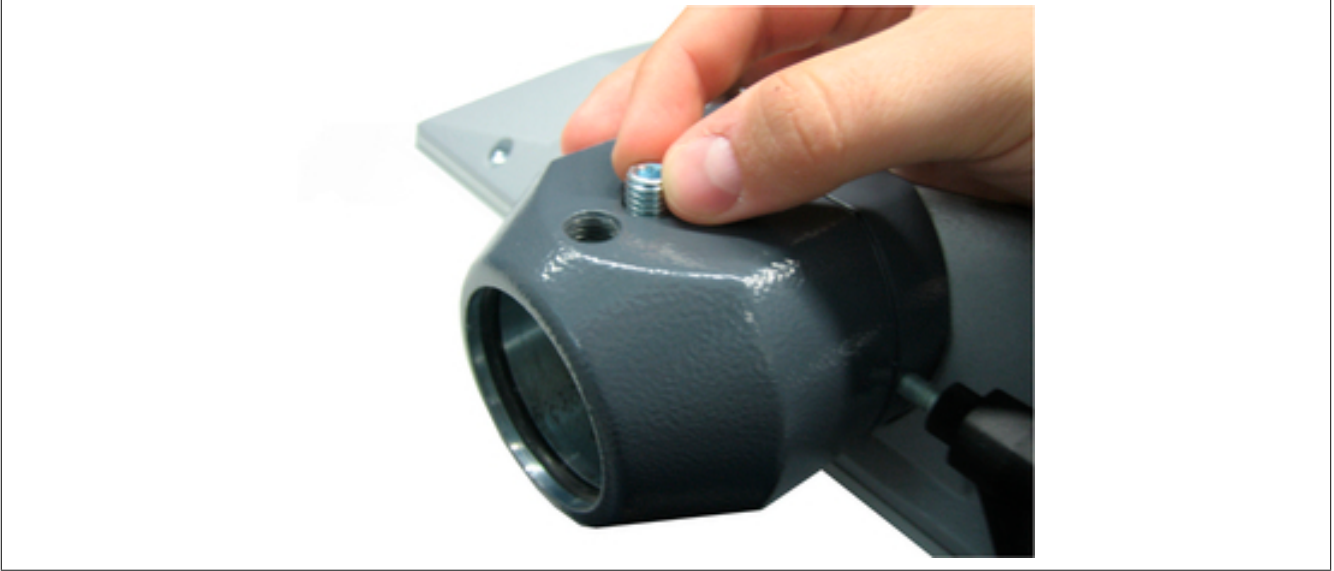
Figure 23: Mounting the screws on the flange
