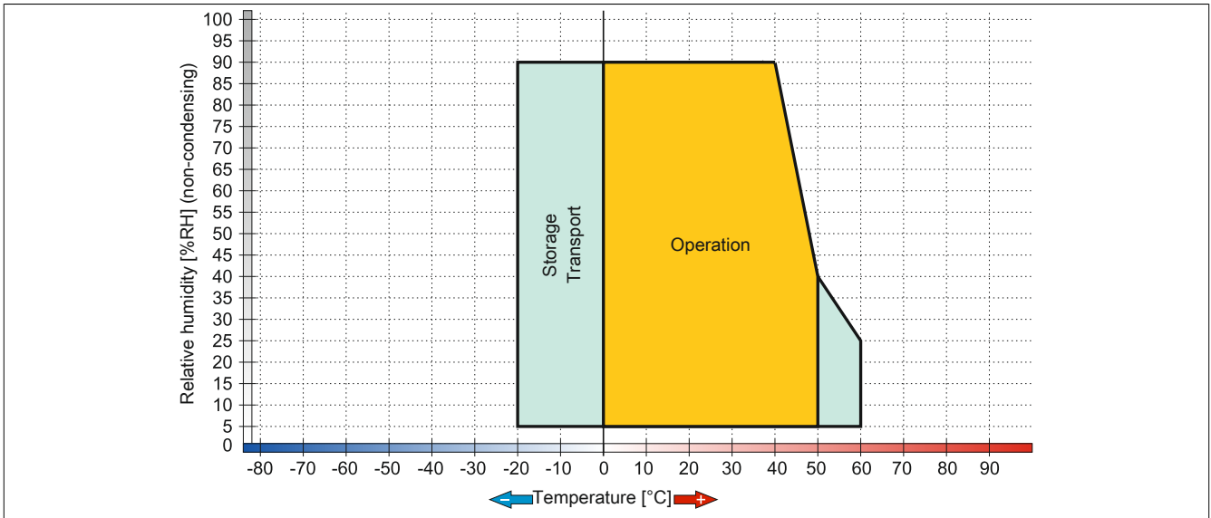
Figure 11: 5PC725.1505-01 - Temperature/Humidity diagram
