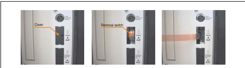
Figure 253: Battery removal
