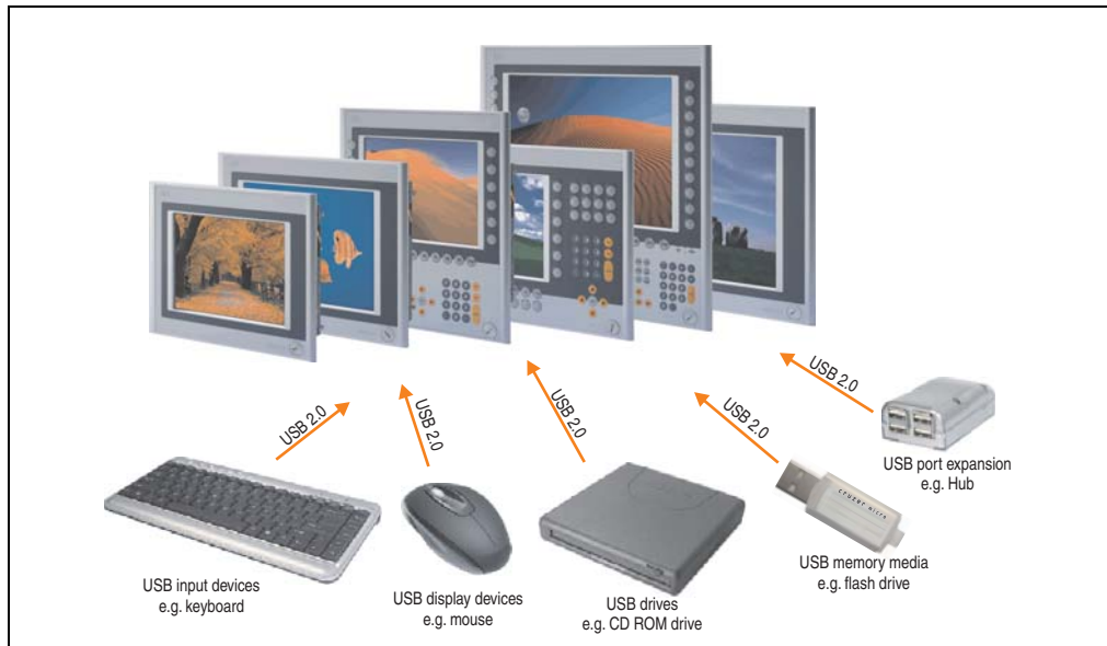
Figure 124: Local connection of USB peripheral devices on the PPC 700
