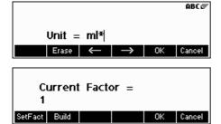
Press the **«SetUnit»** softkey and enter the abbreviation of the custom unit. Confirm by pressing **«OK»**.
