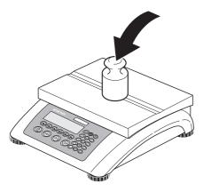
After choosing the calibration weight, place the weight on the weighing pan and then press the  ${}^{\diamond}$ **OK** ${}^{\diamond}$  softkey.
