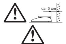
If the **power cord** is damaged, the scale must no longer be operated. Therefore check the cable regularly and ensure that a free space of about 3 cm is left at the rear of the scale, so that the cable is not kinked too severely.
