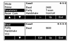
The current Baud Rate, Parity and Handshake settings are displayed on the screen.
