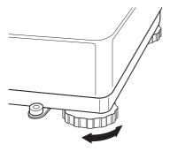
Turn the adjustable feet so that the scale is horizontal. If a spirit level is filled, the bubble must be located within the inner circle.
