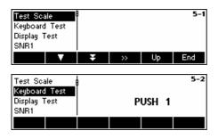
In order to check if all the keys are functioning properly, press **«Yes»** to start the keyboard test.
