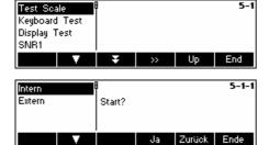
Press « >>> » to enter the settings for the scale test.
