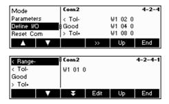
Go to "Vision Setup  $\rightarrow$  COMMUNICATION  $\rightarrow$  COM X  $\rightarrow$  Define I/O and then press «  $\rightarrow$  » to change settings for the I/O relay box.
