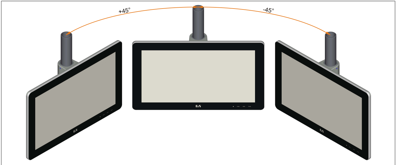
Figure 41: Mounting orientation / Angle of rotation
