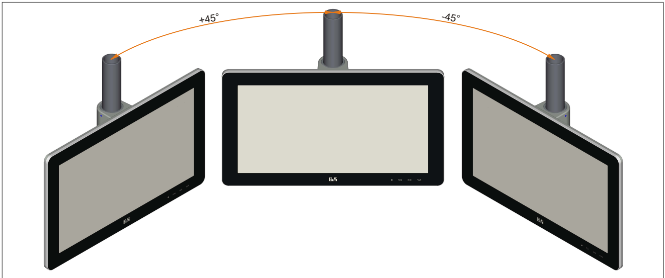
Figure 59: Mounting orientation / Angle of rotation
