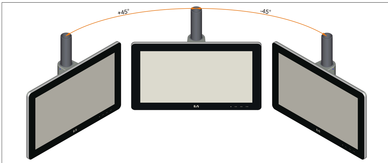
Figure 29: Mounting orientation / Angle of rotation
