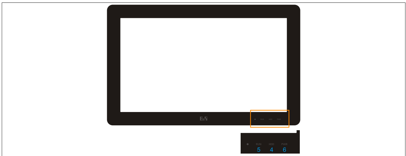
Figure 70: 5AP830.215C-00 / 5AP830.215C-01 - Key and LED configuration
