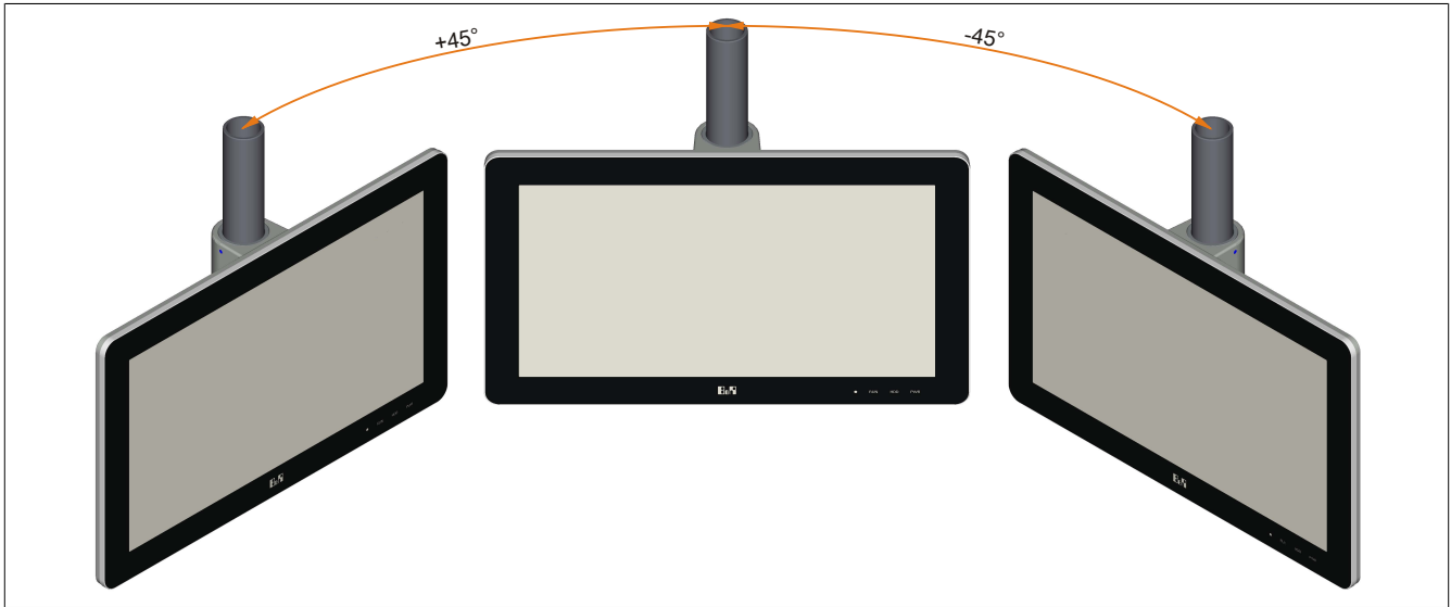
Figure 11: Mounting orientation / Angle of rotation
