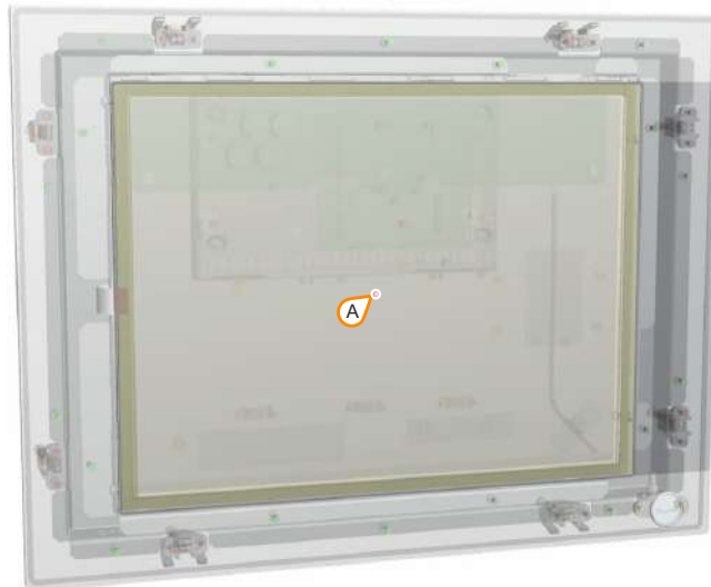
Figure 3: Automation Panel 1000 - Temperature sensor position
