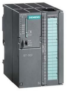
SIPLUS S7-300 CPU 312C for medial exposure -25...+70  $^{\circ}$ C based on 6ES7312-5BF04-0AB0 . Compact CPU with MPI, 10 DI/6 DQ, 2 high-speed counters (10 kHz) Integr. power supply 24 V DC, work memory 64 KB, Front connector (1x 40-pole) and Micro Memory Card required
