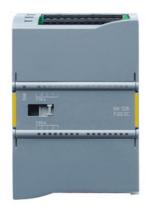
SIPLUS S7-1200 SM 1226 F-DQ 4x24VDC based on 6ES7226-6DA32-0XB0 with conformal coating, -25...+55  $^{\circ}$ C, F-DQ 4x DC 24V 2A, PROFIsafe, 70 mm width, up to PL e (ISO 13849-1)/ SIL3 (IEC 61508)
