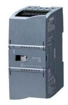
SIPLUS S7-1200 SM 1232 T1 rail based on 6ES7232-4HD32-0XB0 with conformal coating, -25...+60 °C, OT1 with ST1/2 (+70 °C für 10 minutes), S7-1200, analog output, SM 1232, 4 AQ, +/-10 V, 14-bit resolution, or 0-20 mA, 13-bit resolution:
