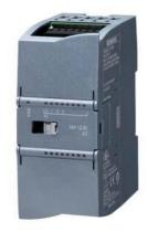
SIPLUS S7-1200 SM 1231 8Al based on 6ES7231-4HF32-0XB0 with conformal coating, -20...+60 °C, analog input SM 1231, 8 Al, +/-10 V, +/-5 V, +/-2.5 V, or 0-20 mA/4-20 mA, 12 bit+sign or (13 bit ADC)
