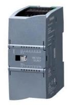
SIPLUS S7-1200 SM 1223 8DI/DQ based on 6ES7223-1QH32-0XB0 with conformal coating, -20...+60  $^{\circ}$ C, SIMATIC S7-1200, digital inputs/ output SM 1223, 8 DI AC/8 DQ RLY, 8 DI 120/230 V AC, 8 DQ relay 2 A
