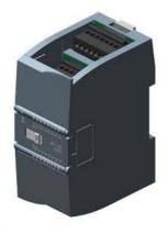
SIPLUS S7-1200 SM 1223 8DI/8DQ based on 6ES7223-1BH32-0XB0 with conformal coating, -20...+60 °C, digital input/output 8 DI/8 DQ, 8 DI 24 V DC, sink/source, 8 DQ, transistor 0.5 A
