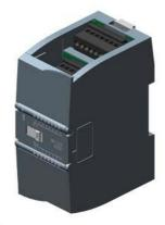
SIPLUS S7-1200 SM 1223 8DI/8DQ based on 6ES7223-1BH32-0XB0 with conformal coating, -40...+70 °C, start up -25 °C, digital input/output SM 1223, 8 DI/8 DQ, 8 DI 24 V DC, sink/source, 8 DQ, transistor 0.5 A
