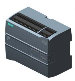
SIPLUS S7-1200 CPU 1215C DC/DC/DC -40...+70°C with conformal coating based on 6ES7215-1AG40-0XB0 . compact CPU, DC/DC/DC, 2 PROFINET ports, onboard I/O: 14 DI 24 V DC 10 DO 24 V DC 0.5 A 2 AI 0-10 V DC, 2 AO 0-20 mA DC, Power supply: DC 20.4-28.8V DC, Program/data memory 125 KB
