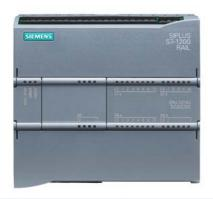
SIPLUS S7-1200 CPU 1214C DC/DC/DC T1 rail based on 6ES7214-1AG40-0XB0 with conformal coating, -25...+60 °C, OT1 with ST1/2 (+70 °C für 10 minutes), compact CPU, DC/DC/DC, onboard I/O: 14 DI 24 V DC; 10 DQ 24 V DC; 2 AI 0-10 V DC, power supply: 20.4-28.8 V DC, program/data memory 75 KB
