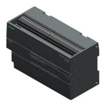
SIMATIC S7-200 SMART, CPU ST60, CPU, DC/DC/DC, onboard I/O: 36 DI 24 V DC; 24 DO 24 V DC; power supply: DC 20.4 - 28.8 V DC, program/data memory 50 KB
