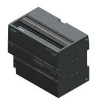
SIMATIC S7-200 SMART, CPU ST40, CPU, DC/DC/DC, onboard I/O: 24 DI 24 V DC; 16 DO 24 V DC; power supply: DC 20.4 - 28.8 V DC, program/data memory 40 KB web server support
