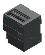
SIMATIC S7-200 SMART, CPU ST20, standard CPU, DC/DC/DC, onboard I/O: 12 DI 24 V DC; 8 DQ 24 V DC; power supply: DC 20.4 - 28.8 V DC, program/data memory 20 KB web server support
