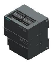
SIMATIC S7-200 SMART, CPU SR20, CPU, AC/DC/relay, onboard I/O: 12 DI 24 V DC; 8 DQ relay 2A; power supply: AC 85 - 264 V AC at 47-63 Hz, 77 to 138 V DC program/data memory 20 KB
