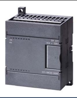
SIMATIC S7-200, T/C INPUT MOD. EM 231, FOR S7-22X CPU ONLY, 4 AI, +/-80 MV AND THERMOCOUPLE TYPE J,K,S,T,R,E,N; 15BIT+VORZ.
