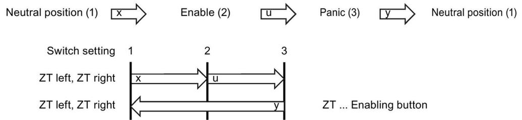
If the operator has pressed the enabling button through to the "Panic" setting, the "Enable" setting will be skipped when the switch is released.
