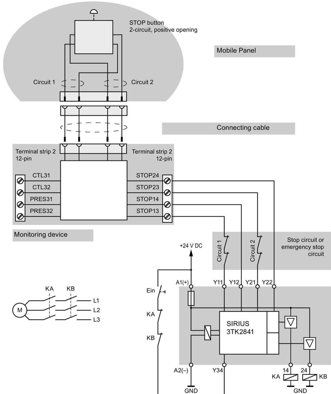
All contacts of the safety relay (contactor) KA and KB are fitted with positively-driven contacts in accordance with EN 50205:2002.
