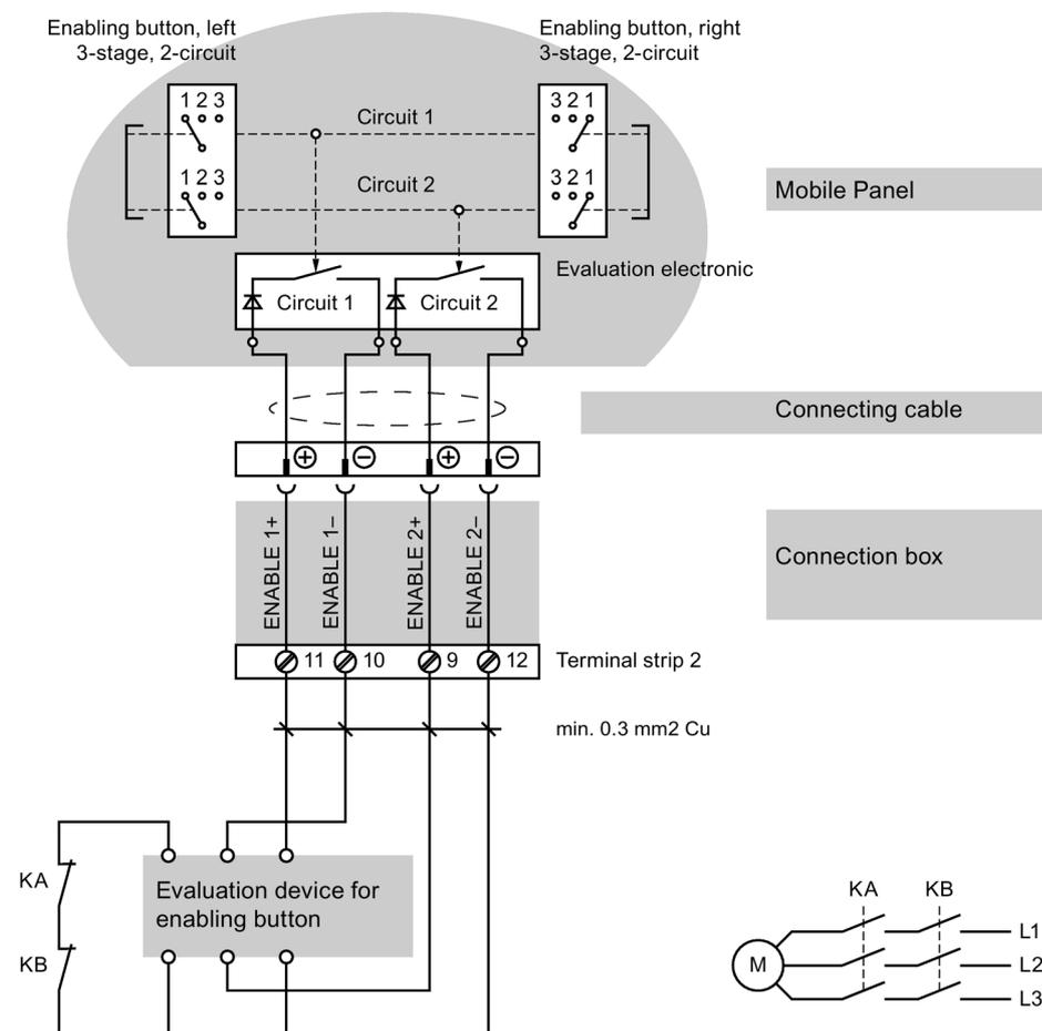
10.6 Wiring examples for enabling button and stop button
