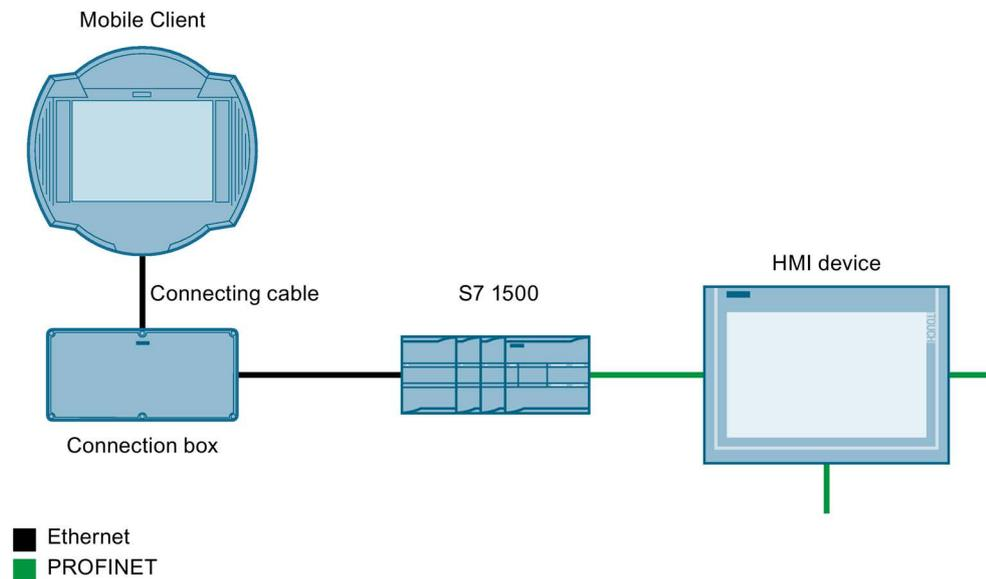
The HMI device is used for monitoring or controlling the operating process. The controller in turn supplies the results of the operating process, which are displayed on the Mobile Client.
