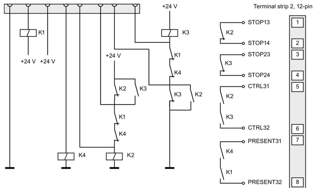
Mobile Client plugged, power supply switched on and STOP inactive
