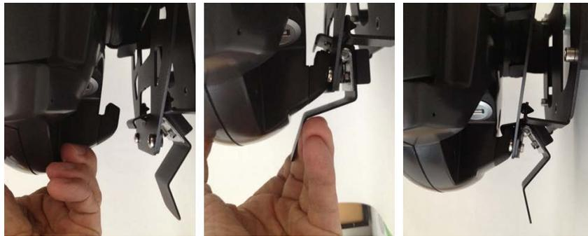
The device will slide into the lock position.
