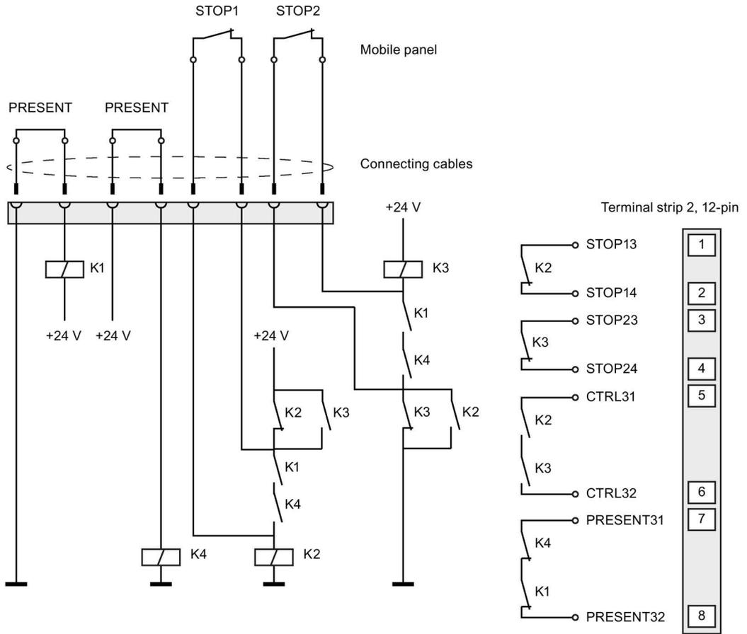
Mobile Client plugged, power supply switched on and STOP active
