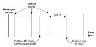
As can be seen from the diagram, the actual time from network loss to Unidrive trip will range from #20.11 ms to 2  $^{*}$  #20.11 ms. If the trip time is set too low, spurious network loss trips may be seen.
