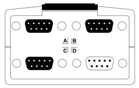
The Profibus-DP connectors are parallel connectors, so either connector can be used. The pin-out connections are identical, and are given in the table below.
