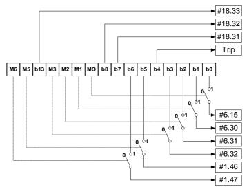
If mask bits M0 and M1 are set to 1, ENABLE and RUN FWD are updated with the values of b0 and b1 (either 0 or 1) every time the control word value is received. JOG and RUN REV will not be updated, even if the values of b2 and b3 change, because their mask bits (M2 and M3) are not set to 1. If M0 and M1 are reset to 0, the values in b0 and b1 will NOT be written to ENABLE and RUN FWD, and these parameters will remain set to their current state.
