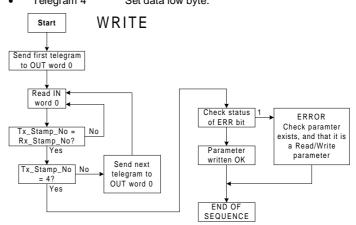
The following example telegrams show how to write a value of 120.0 Hz (0x04B0) to #1.21 in the Unidrive.
