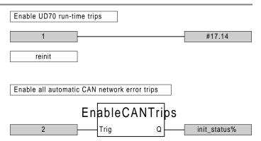
By setting #17.14 to 1 and executing the REINIT command, this will force the UD70 to read the UD70 configuration parameters (#17.PP) again, and enable the UD70 run-time trips.
