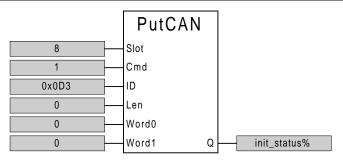
To receive a message from the CAN network, a slot must be configured with a mask for the CAN ID. If a message is received by the CAN controller, with an identifier that matches the mask of one of the slots, the message is put into that slot. Otherwise, the CAN controller discards the message.
