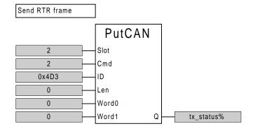
Use CANSTATUS and GETCAN to detect and retrieve the RTR response frame. (See section 6.5). Usually, only one slot needs to be allocated to receive RTR response frames, as the slot mask can be re-configured with the appropriate CAN identifier before the RTR frame is actually sent.
