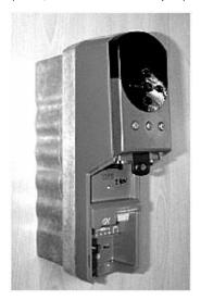
To remove the UD70, pull firmly on the black tab, and the module will disengage from the connector.
