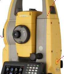
Built-in laser plummet is equipped for quick instrument setting. 5 brightness levels are ready for optimum visibility. (option)
