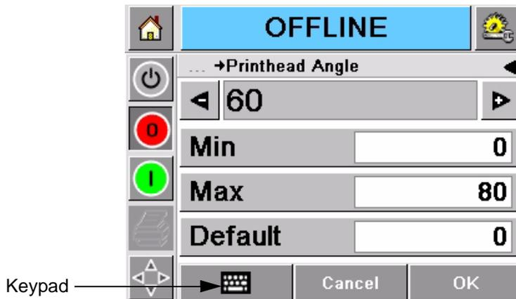
Figure 4-18: Adjust Printhead Angle
