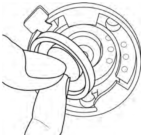
Figure 8.9 Removing the membrane
