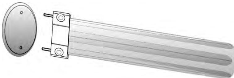
Figure 8.1 Removing the filter covers
