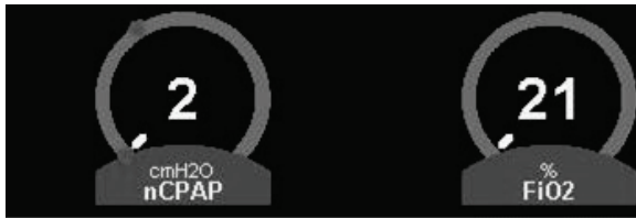
Figure 6-6: nCPAP Primary Controls and Alarm Threshold Indicators
