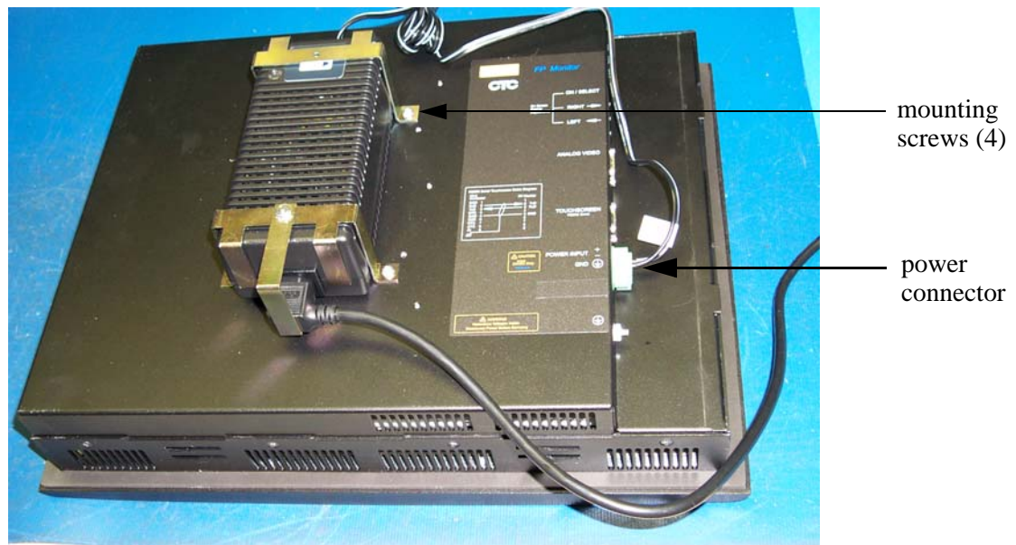
Figure 2-2: Mounting an External AC Adapter
