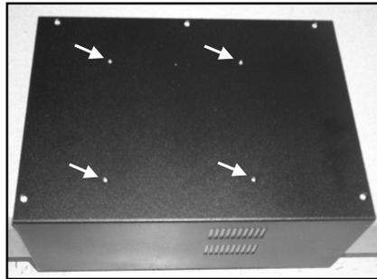
3. Attach the floppy drive to the rear of the workstation using the predrilled holes in the workstation and the four screws provided. Test access with a floppy disk.
