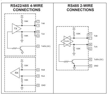
Note: All Parker - SSD Drives devices connect A to A and B to B.
