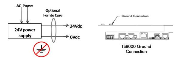
**Important:** Do not connect the power supply common to ground. The TS8000 has its own chassis ground that should be utilized. To further reduce electrical noise, SSD Drives also recommends the use of a ferrite core on the 24Vdc and 0Vdc leads between the power supply and the TS8000.
