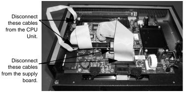
9. Disconnect the four ribbon cables shown below.
