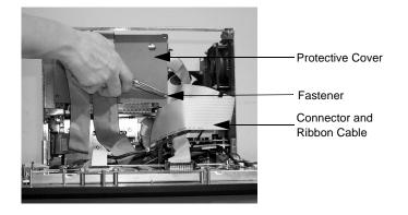
10. Use a pair of needle nose pliers to squeeze the fasteners that hold the protective cover to the CPU Board. See the illustration below.
