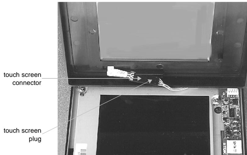
5. Locate pin 1 on the touch screen plug, and align it with pin 1 of the new touch screen connector. A “1” identifies pin 1 on the touch screen plug.
