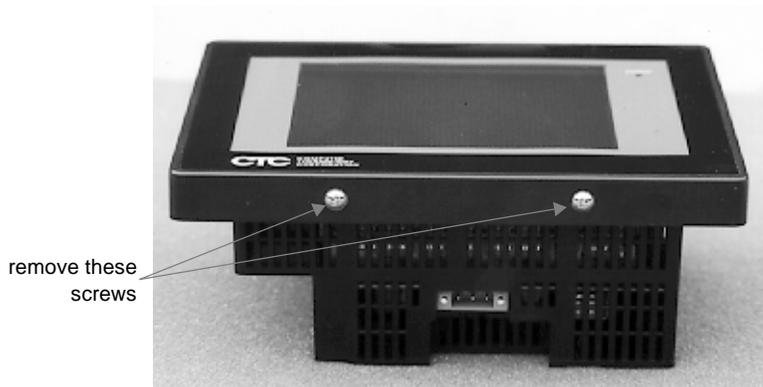
3. Carefully lift the bottom of the touch screen approximately two inches while disengaging the tabs that secure the touch screen to the top of the unit.
