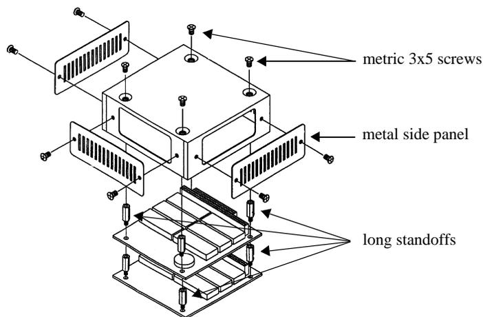
4. Fasten a second set of the longer standoff screws onto the second PC/104 card.
