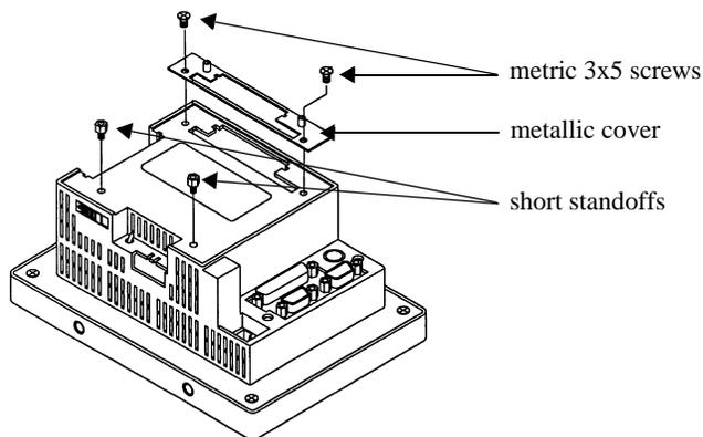
This will expose the PC/104 connector and the two pre-installed standoffs on the metallic cover.
