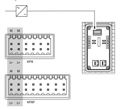
The figure below shows the connection between KP32F and the power supply.
