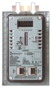
When installed, the labeling strips can be inserted if the mounting has a material thickness of < 3.5 mm. With larger material thicknesses, the disassembly of the HMI device is required if a labeling strip should be changed.
