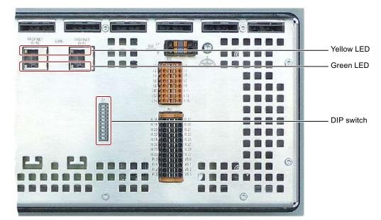
The following control elements and displays are located on the rear of the KP32F.
