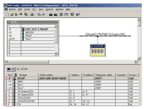
Parameters for following slots are entered in the HW Config for the KP32F:
