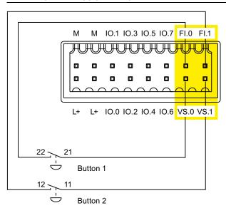
Observe the respective setting for "Evaluation of the sensor" in HW Config - see section "Setting the fail-safe properties (Page 89)".
