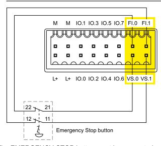
The EMERGENCY-STOP button must be connected as an equivalent break contact. Observe the affiliated setting for "Evaluation of the sensor" in the HW config - see section "KP8F – Setting the fail-safe properties (Page 77)".
