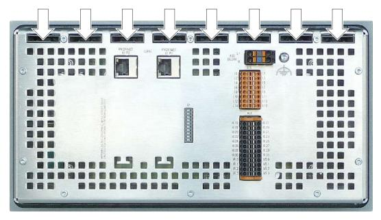
With KP32F you can replace the labeling strips in the installed state without restrictions.
