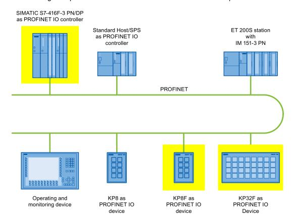
In the example, each PROFINET IO device communicates with just one PROFINET IO-controller. The PROFIsafe device communicates here exclusively with the F-PROFINET IO controller.
