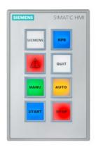
SIMATIC HMI KP8F PN, Key Panel, 8 short-stroke switches with multi-colored LEDs, PROFINET interfaces with PROFIsafe; 8 DI/DO and 2 safety DI pins, 24 V DC can be looped through parameterizable as of STEP 7 V5.5
