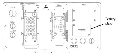
Connector plate on robot base
