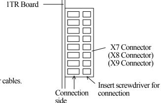
It is recommend to use AWG22-24 or equivalent for cables. (Stripped wire length: 7 mm)
