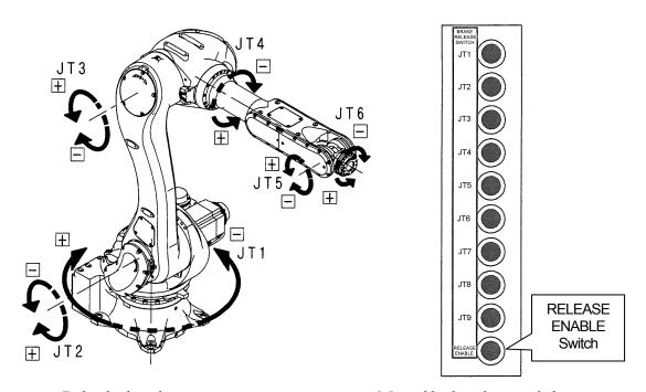
Robot brake release axes
