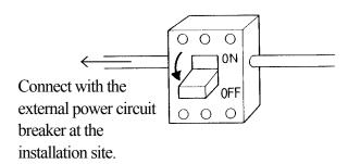
Connect the external power according to the following procedure.
