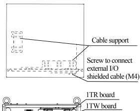
Use cable support for wiring of 24 Vdc or less such as I/O, Ethernet and fieldbus cable etc. Make sure not to put any stress on connectors on each board.
