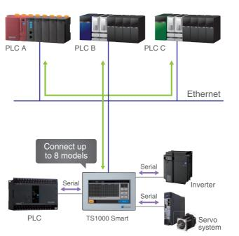
\* With TS1070S, up to 3 models can be connected.
