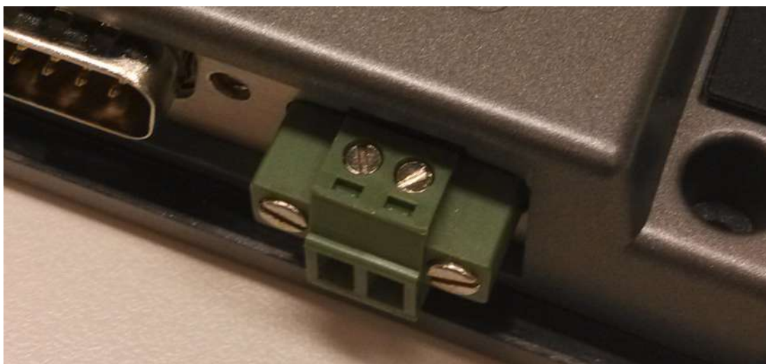
Figure 2.3 Power Line into the Power Receptor
