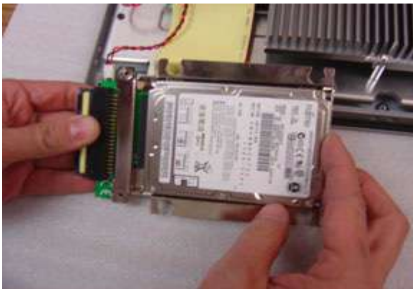
Figure E.6: Installing the HDDr
