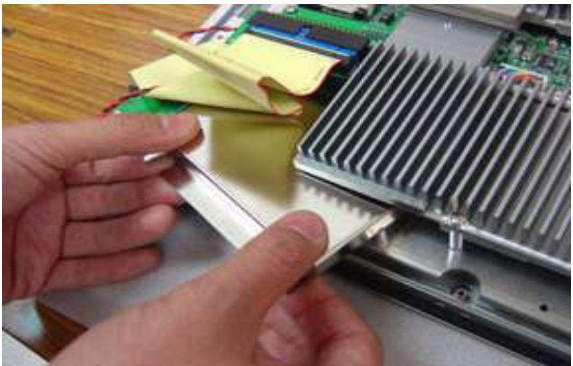
Figure E.4: Pulling out the HDD bracket
