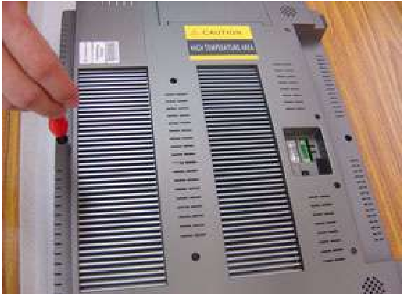
Figure E.15: Reinstalling the Rear Cover
