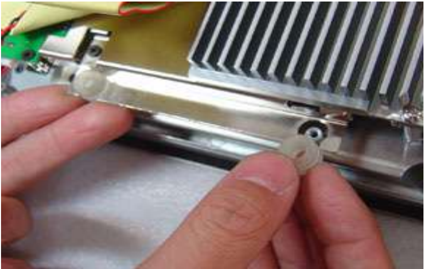
Figure E.3: Removing the HDD kit
