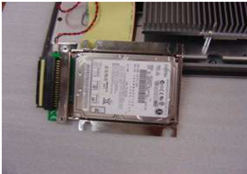
Figure E.7: Linking the HDD with the Connector
