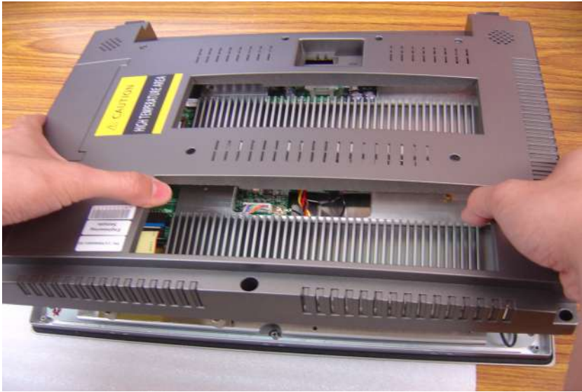
Figure E.1: Removing the Rear Cover
