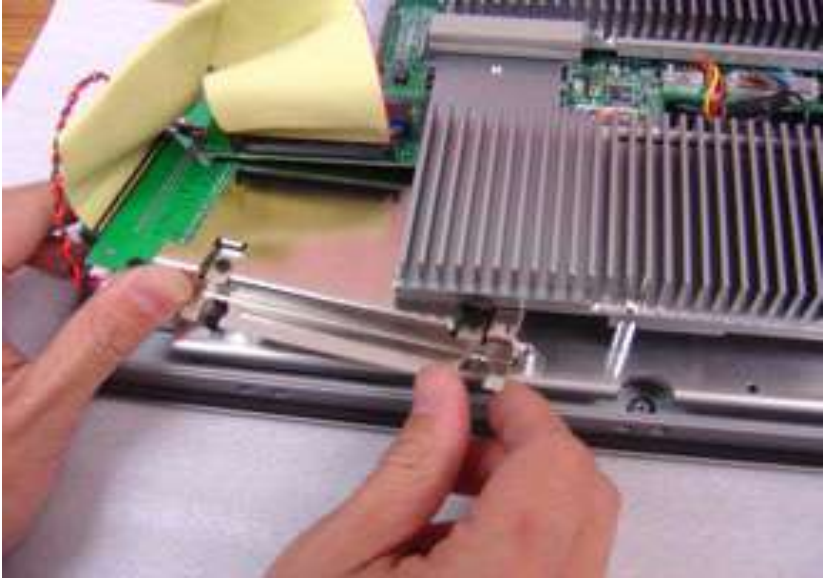
Figure E.11: Sliding the HDD Into Position
