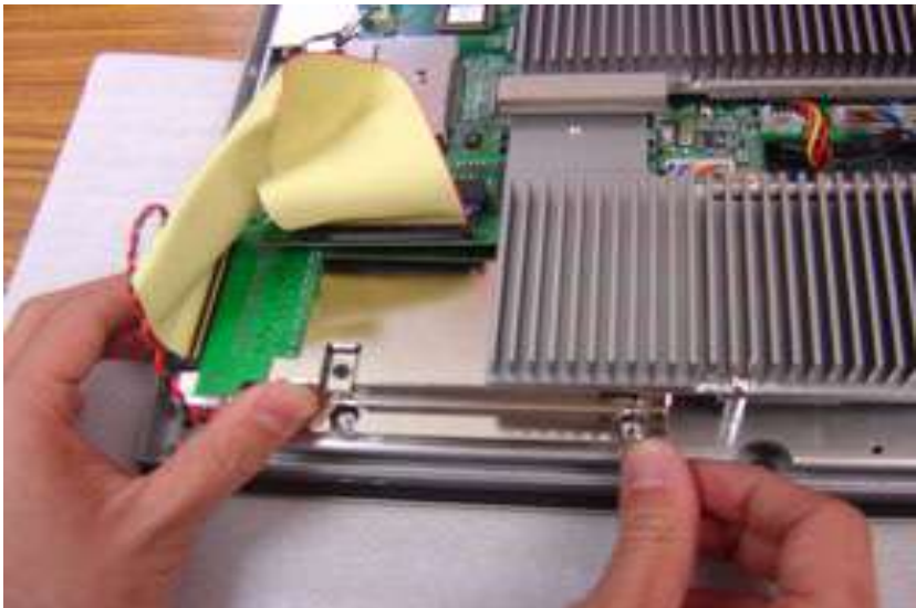
Figure E.12: Completed HDD Installation
