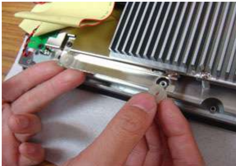
Figure E.13: Mounting the Rubber Cushions
