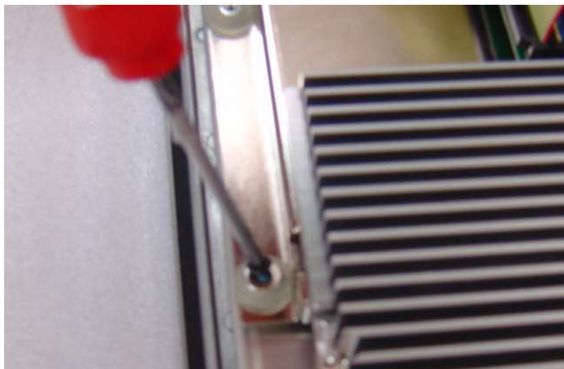
Figure E.14: Fastening the HDD Module
