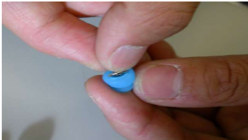
Figure E.15: Placing a screw into its rubber casing
