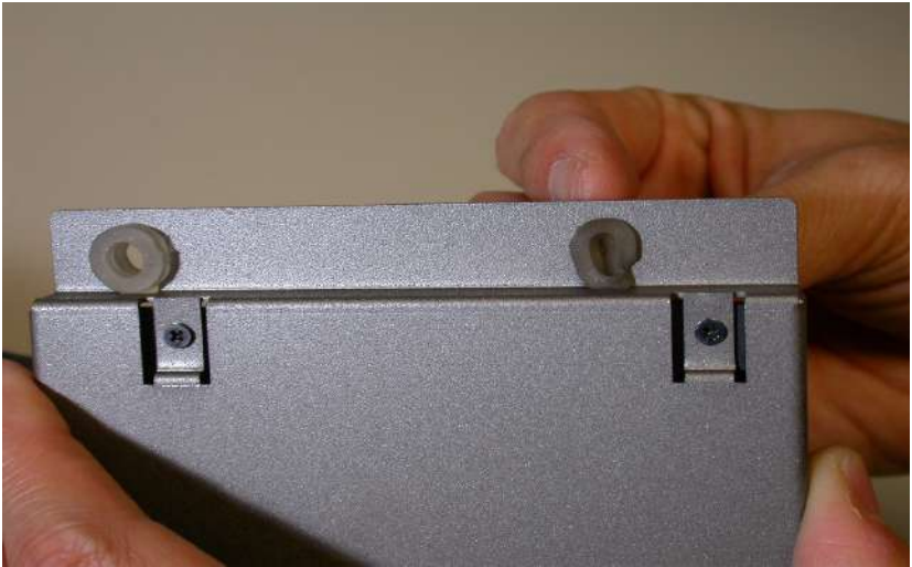
Figure E.10: Mounting the cushions - 2
