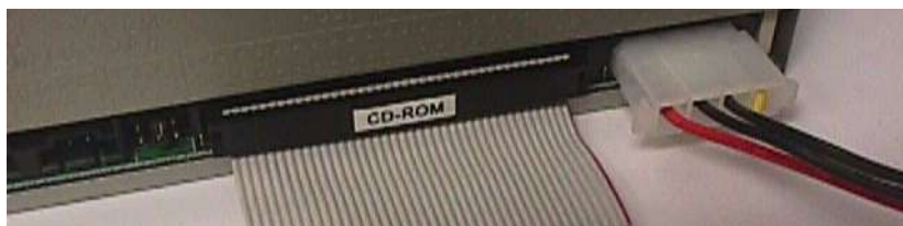
Figure D.7: Plugging in the CD-ROM Drive
