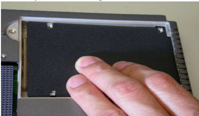
Figure E.19: Laying in the HDD insulator
