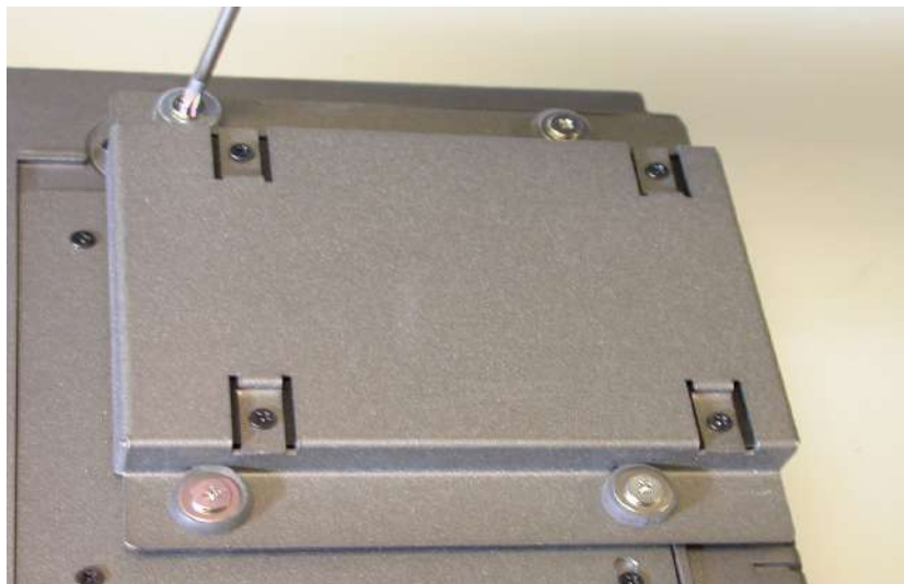
Figure E.13: Fastening the HDD holder
