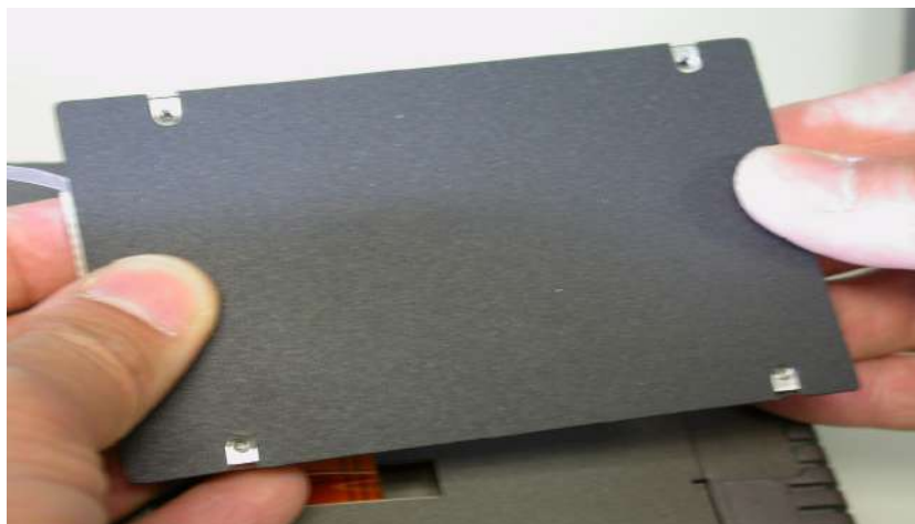
Figure E.6: Placing the HDD insulator on the HDD
