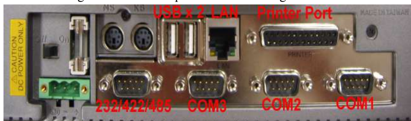
Figure 1.1: I/O Port Arrangement
